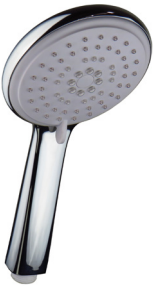
C28140 Handshower Massage, Wide, Champagne Self cleaning (anti-limescale) This handshower comes with multi spray functions and each time you change the sprays to massage or champagne, the internal mechanism will be activated to clean the nozzles.
